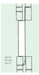
piece ready to receive the circular window. It fits snugly around the window frame, providing a 360° barrier. The circular window is immediately enveloped in a durable cavitray thus ensuring correct and thorough protection. The inside skin of the cavity wall and the sides of the circular window frame are protected from dampness.
